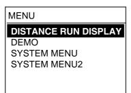
Press the Omnipad at ▲ or ▼ to select a menu item (current selection is highlighted) and press the [ENT] key. For example, when DISTANCE RUN DISPLAY is selected the following display appears. Distance run is a form of contact closure, 200 pulses/nm. To select IEC 61162 sentence, see paragraph 1.6.1.
