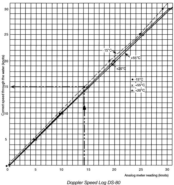
ANALOG DISPLAY UNIT CORRECTION DIAGRAM AT EXTREME TEMPERATURES
