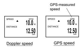
"AUTO" position indicates a Doppler speed (SDME) but if the DS-80 fails, a GPS speed will be indicated.
