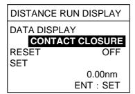
Press the Omnipad at ▲ or ▼ to select the menu item desired and press the [ENT] key. For example select RESET.
