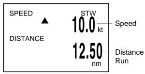
**Note:** STW means Speed Through Water. This indication flashes when transducer temperature, which can be monitored on the TEST display (see page 16), is abnormal. This means speed accuracy is less than stated in the specifications.
