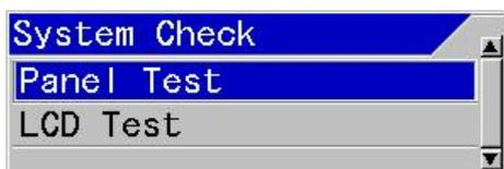
4. When panel test or confirmation of system status is performed, select [Panel Test] with
