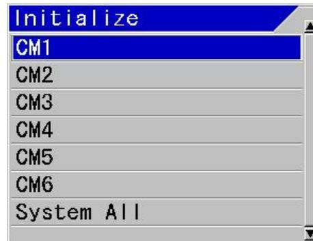
4. When an specified CM is to be initialized, select [CM1] to [CM6] with [▲] and [▼] keys. To initialize the whole system, select [System ALL].
