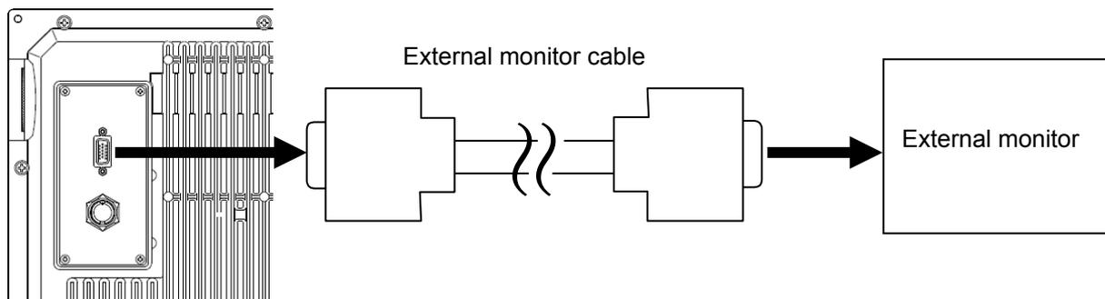
Fig. 1.30 Connection of External Monitor-2
