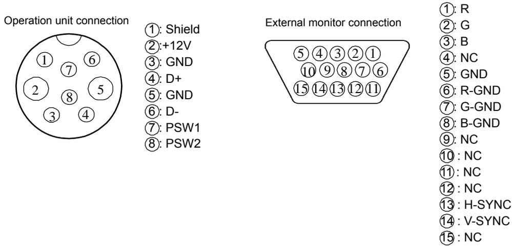
Fig. 1.21 Pins assignment of rear connector-2
