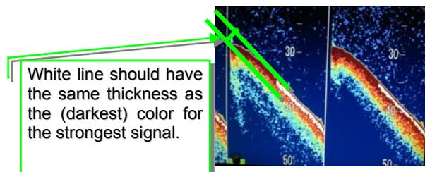
5. Pressing the gain knob at the side to be adjusted a few times, move to the position of the Gain (TD) box to be adjusted. (the red mark at right top side will move)
