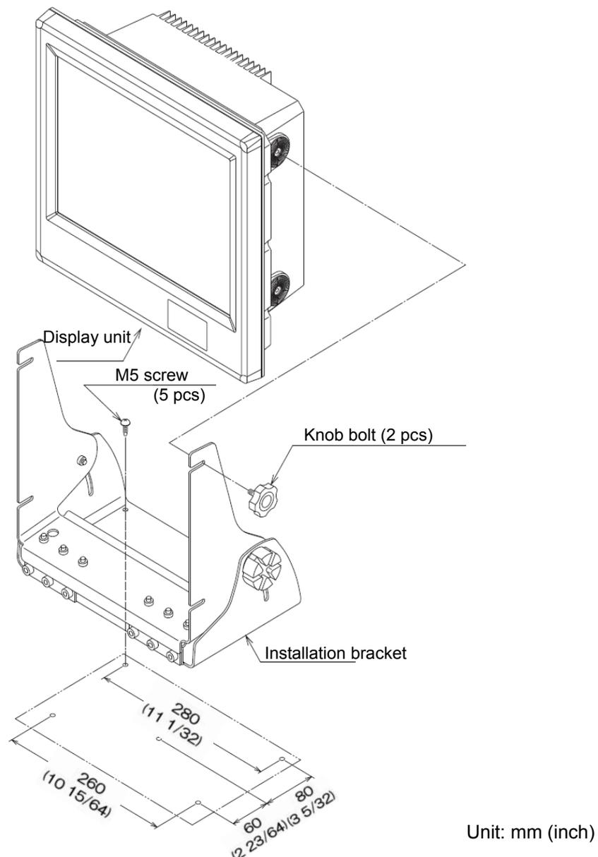
**Fig. 1.2 Desk-top installation of Display unit**
