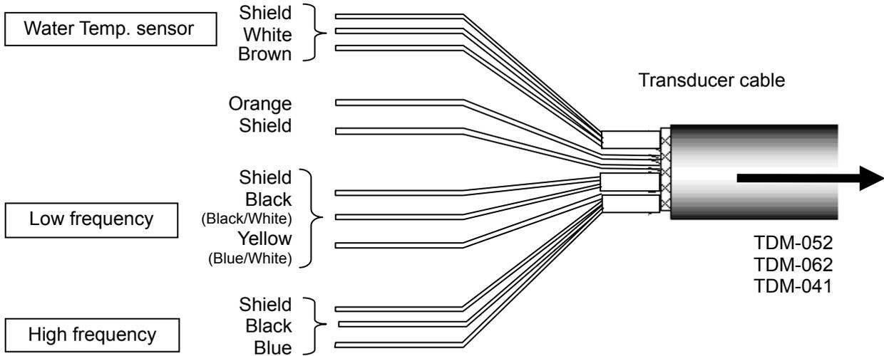
Fig. 1.25 Details of transducer cable
