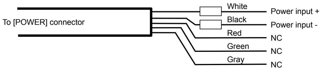
Fig. 1.22 Connection of DC power cable
