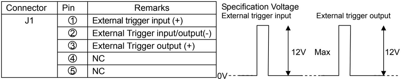
Fig. 1.27 External trigger
