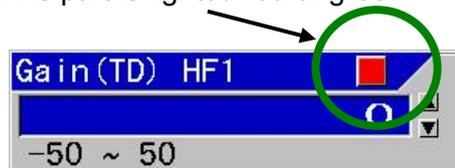
The gain (TD) setting shall be adjusted in such a way that the white line in sea bottom has the same thickness as that of the strongest signal color area.
