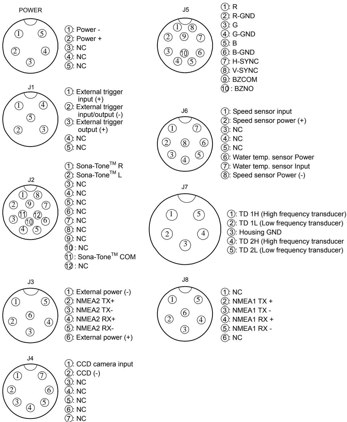
**Fig. 1.20 Pins assignment of rear connector-1**
