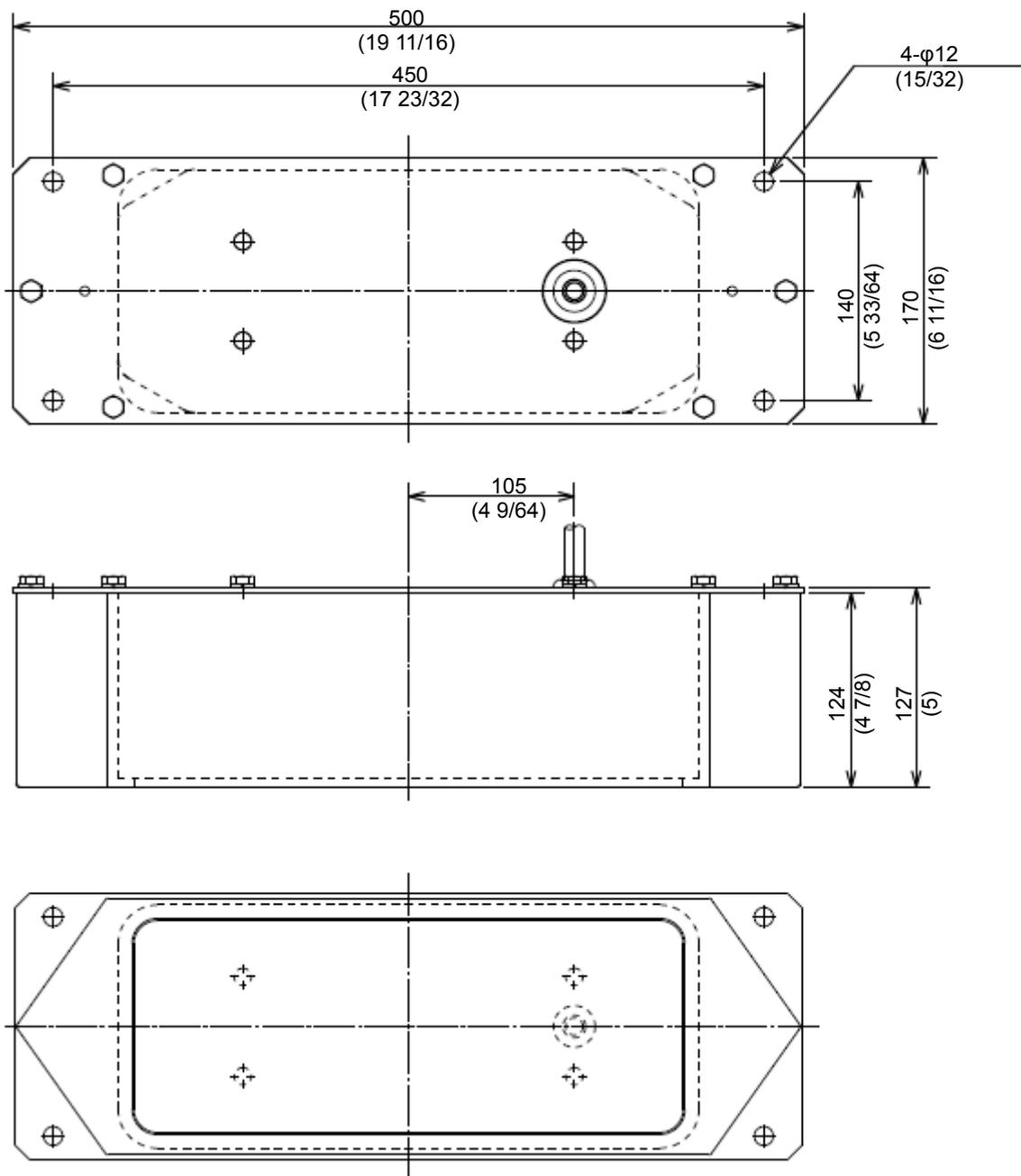
**Fig. 1.16 Outline view of the unit on FRP and wooden boat**
