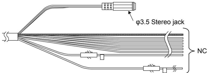
Fig. 1.28 Connection of External Speaker for Sona-Tone™
