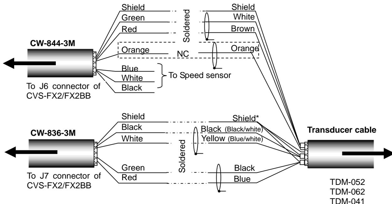
**Fig. 1.23 Connection of transducer cable**
