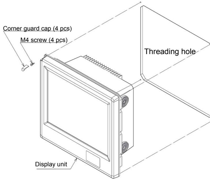
**Fig. 1.4 Flush-mount installation**
