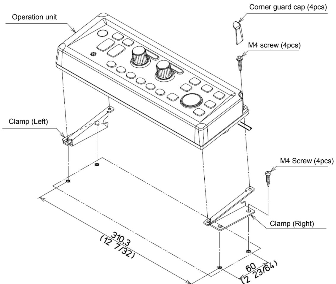
Fig. 1.7 Desk-top installation of Operation unit
