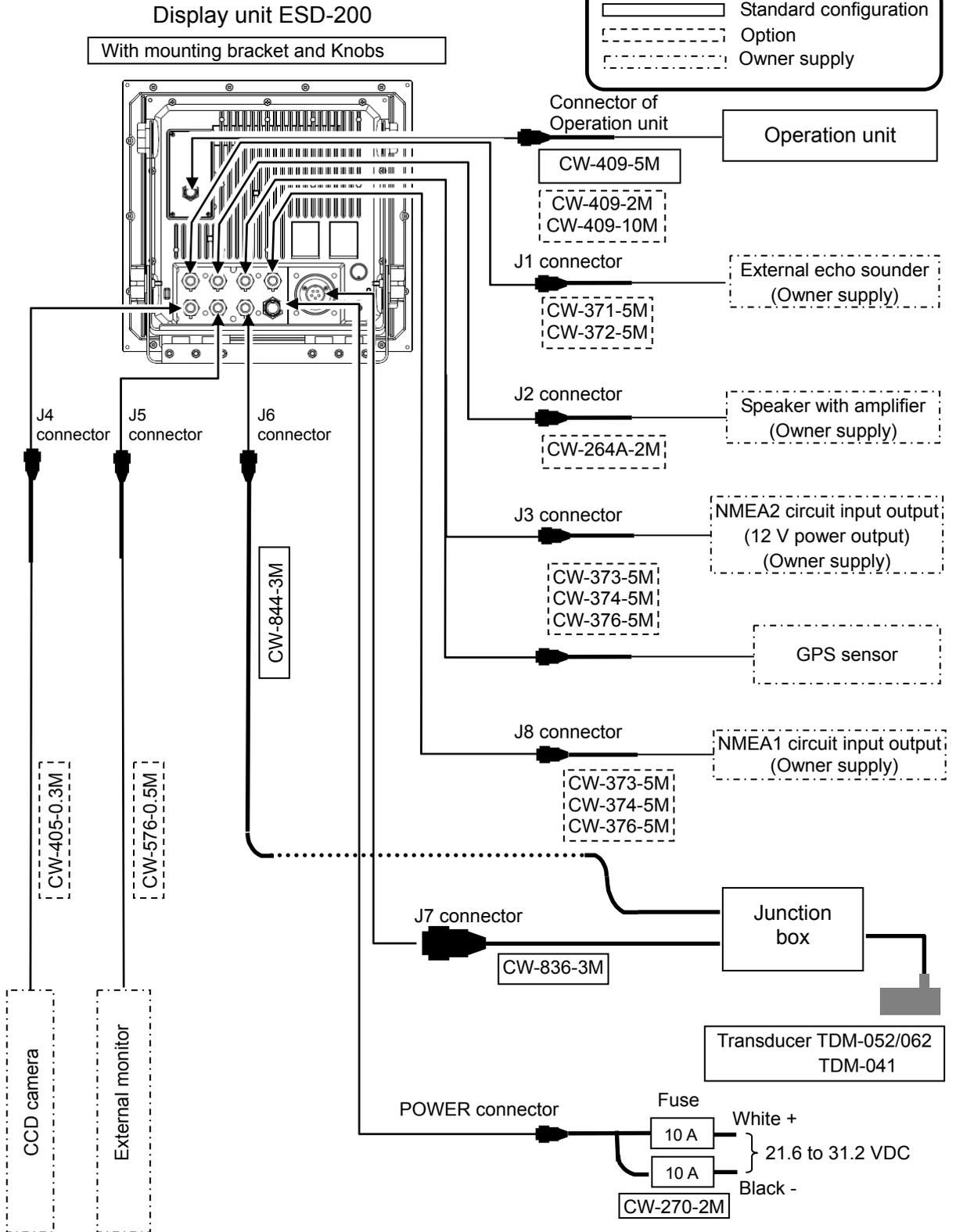
Connection diagram of CVS-FX2BB
