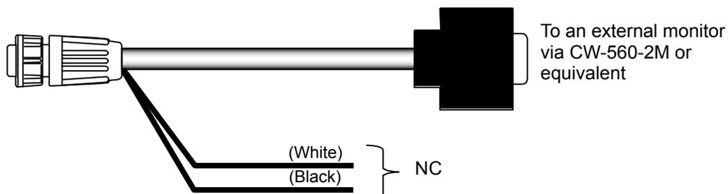
Fig. 1.29 Connection of External Monitor-1
