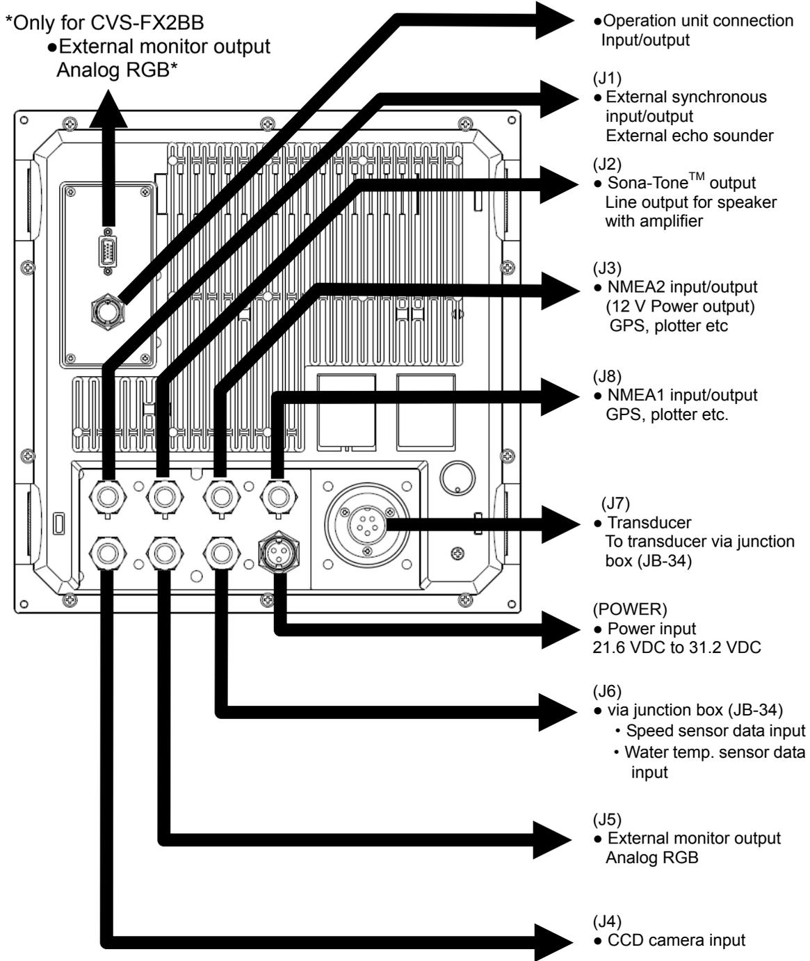
**Fig. 1.19 Cable connections**
