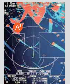
Zoom box tracks the target object according to its movement.
