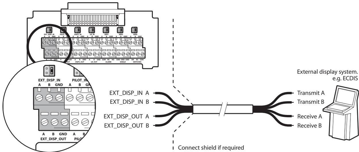
Figure 45 Example connection to external display equipment
