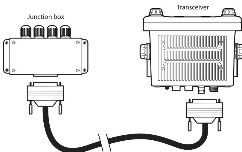
*Figure 43 Connecting the junction box to the transceiver*
