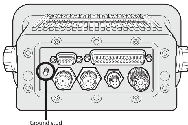
Figure 49 Grounding the transceiver
