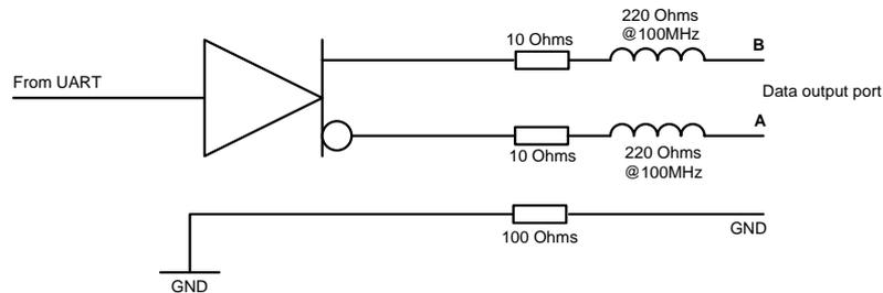
Figure 57 Data output port schematic
