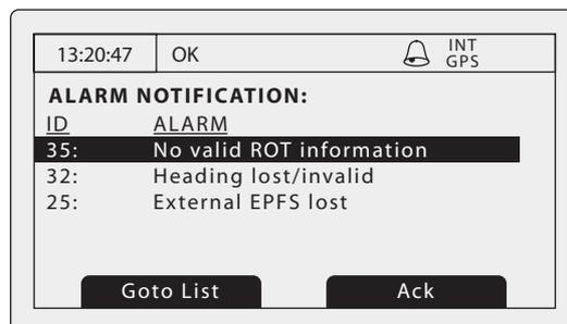
Figure 16 Alarm notification screen
