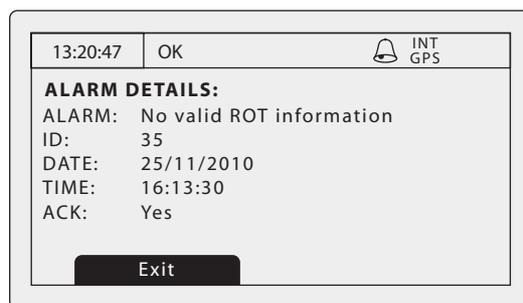
Figure 11 Alarm details view
