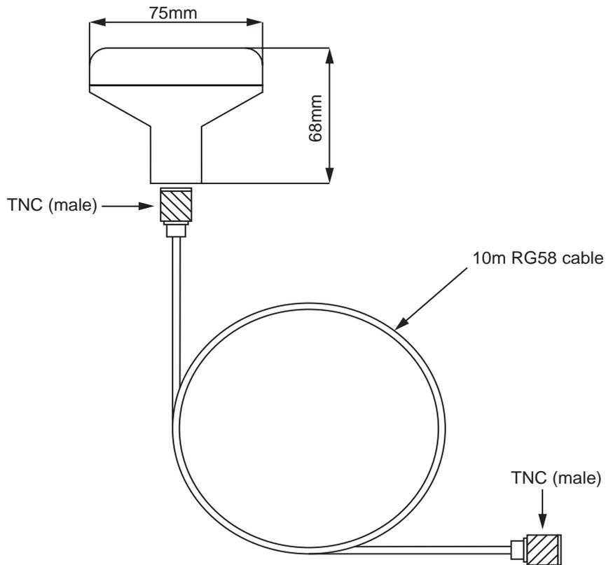
*\* An equivalent alternative GPS antenna may be supplied with transceiver variants without the dual mode internal GNSS receiver. The dimensions of the supplied antenna may vary from those shown here.*
