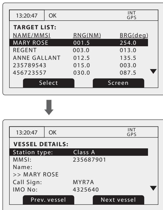
Figure 5 Target list screen and vessel details view
