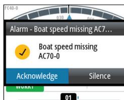
The most recent alert is acknowledged by pressing the rotary knob. This removes the alert notification, and silences the alert from all units that belong to the same alert group. A reminder reappears at given intervals for as long as the alert condition exists.
