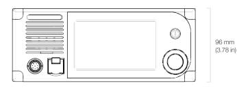
240 mm \*Flushmount cut out (9.44 in) 215 mm x 89 mm
