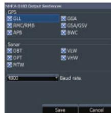
You can also adjust the Baud rate, but the default setting works best under most conditions.
