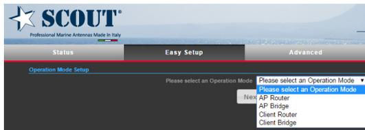
**AP Router** - Connect Ethernet port to a broadband Modem. All devices then connect via WiFi just like a regular wireless Router.
