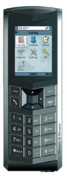
When connected to the terminal the IP handset provides a dedicated BGAN menu with a subset of the terminal configuration options.
