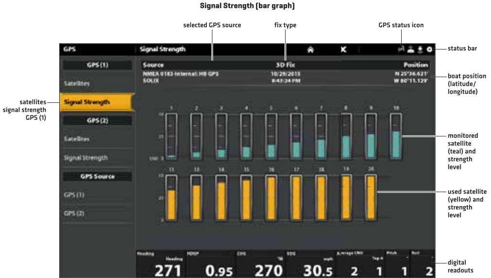
Signal Strength (GPS 1/GPS 2): displays vertical bar graphs indicating the satellite signal strengths with the respecting CNO (Carrier-to-Noise) value (0 to 60).
