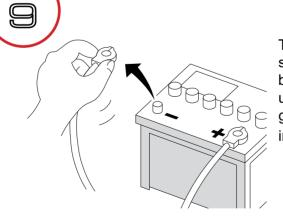
To avoid potential shorts in the electrical system, be sure to disconnect the (–) battery cable before installation. Use this unit with a 12-Volt battery and negative grounding only. Failure to do so may result in a fire or malfunction.
