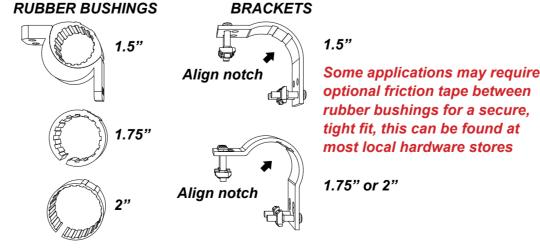
1) Determine the size rollbar for your vehicle, install rubber bushings on rollbar 2) Insert and align notch of rubber bushings into the aluminum brackets 3) Apply supplied Loc-Tight to allen bolt tips, let dry for 20 minutes, then align the allen bolts and T-nuts into the T-channel, firmly tighten 4) Recheck all allen bolts are tight, ensure T-nut's are properly seated in the *T-channel* correctly
