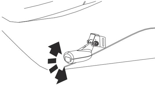
→ **Note:** A transducer that is tilted too far in either direction does not perform well; missing targets, or losing the bottom at speed.
