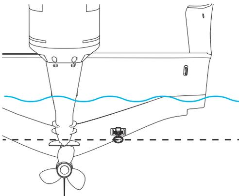
→ **Note:** Ensure the entire bottom surface of the transducer hangs at least 3 mm (1/8th of an inch) lower than the bottom of the hull.
