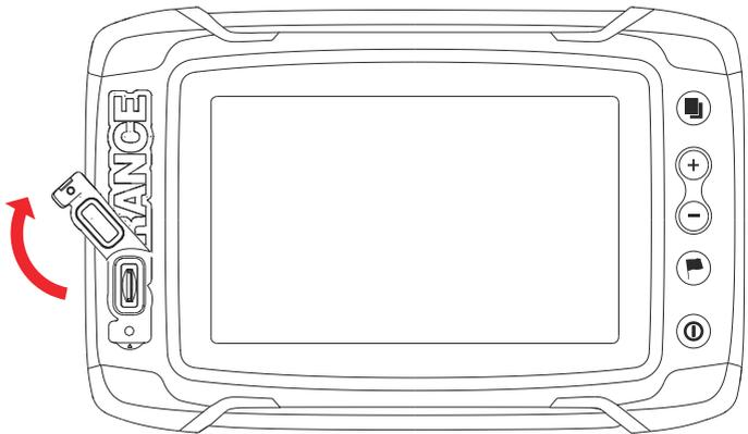
The card reader door should always be securely shut immediately after inserting or removing a card, in order to prevent possible water ingress.
