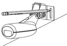
Hold the transducer with bracket up to the transom of the boat and trace the slotted screw hole locations (two on the 83/200 KHz transducer, and four on the 50/200 KHz transducer). Mark drilling points in the middle of each outline, to allow for transducer height adjustment. Drill pilot holes to suit fasteners.
