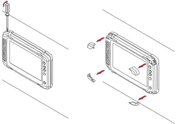
6. Check the fit of the unit, and use a file to remove any remaining obstructions. If water-tightness is required, apply a thin, continuous bead of sealant to the back of the unit prior to final installation. Sealant should be of a *neutral cure* type to prevent damage to the plastics.
