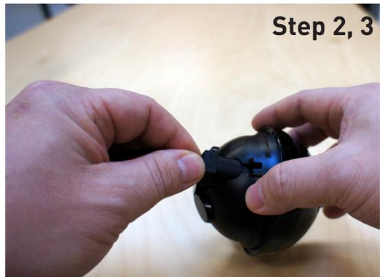
**Step 3:** Push the USB cord into the bottom of the sonar so that it is in snugly. You will notice that you **MUST** slide the charge cord past the transducer on the bottom of the sonar which makes it slightly difficult to get the charge cord into the side of the unit. This is the correct way to ensure a good connection with your sonar.
