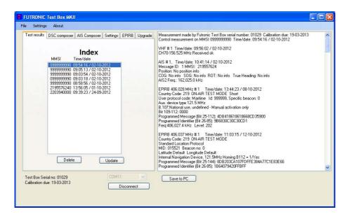
The Futronic MKII comes with free PC software which allows you to view test results and save them to a PC, compose custom-made DSC and AIS messages, generate complete finished EPIRP test reports, personalize test box settings and upgrade the test box with new features.
