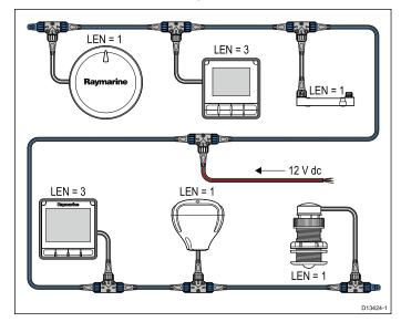
In the example above the system has an overall LEN of 10, so the optimum connection point would be to have 5 LEN either side of the connection point.
