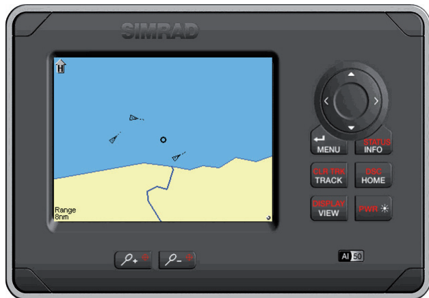
Figure 1.1 - AI50 Class B Transceiver
