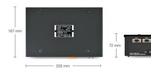
2 video channel input Analog RGB/Hs/Vs Up to 1920 by 1200 pixels Record interval 15sec/image Output to NDV-1900 via LAN Refresh rate 60 to 85 Hz Power 100V to 240V AC (15VA)
