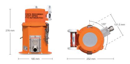
TCP/IP protocol (IEE802.3) 32GB SS drive (48hr record) Operates 90 days after activation Detectable 1800 to 3600m<sup>1</sup> 37.5kHz underwater beacon Temperature: -25° to 55°C Power from NDV-1900
