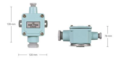
Required for float free capsule between NDH-339 and NDV-1900 Built-in terminal blocks Wall mount installation Temperature: -25° to 55°C Humidity: ≤93% noncondensing Protection rate: IP56
