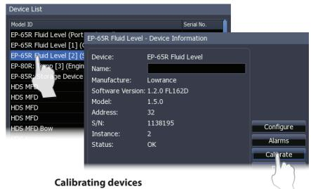
Devices that can be calibrated from the device list will have a Calibrate button on the Device information dialog.
