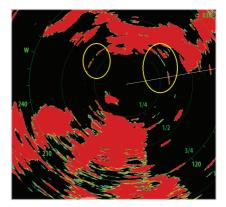
Occasionally false target returns can occur adjacent to strong target returns such as large boats or container ports. This occurs because not all of the transmitted radar energy can be focused into a single beam by the radar antenna, a small amount energy is transmitted in other directions. This energy is referred to as sidelobe energy and occurs in all radar systems.
