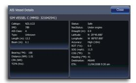
You can display detailed information for a target by activating the menu when the target is selected.
