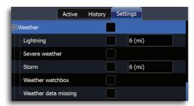
A watchbox is defined by the National Weather Service. When the alarm is turned on you will get an alarm if your vessel is inside or moves into a watchbox. Access the Alarms utility to set up weather alarms
