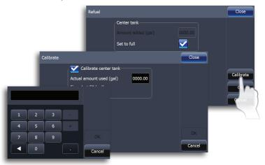
If you add fuel, but do not fill the tank, you must enter the amount of fuel added to the tank to ensure the accuracy of fuel economy calculations
