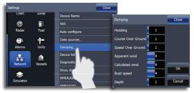
Damping accomplishes this by averaging the data. The higher the damping level, the more data history will be averaged. As a result, higher damping levels cause a delayed response to changes in the data.
