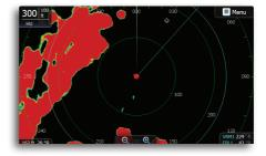
The EBL/VRM is by default positioned from the center of the vessel. It is however possible to offset the reference point to any selected position on the radar image.
