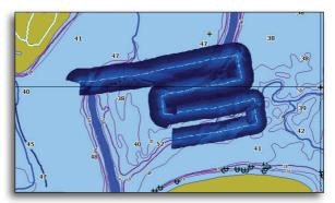
→ **NOTE:** Optimal speed for viewing or logging StructureMap data is between 2-8 mph (3-12 kmh). Live mode is disabled for speeds greater than 10 mph.
