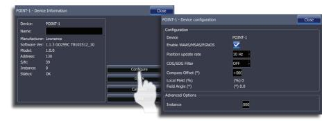
Position update rate may be adjusted (1Hz, 5Hz or 10Hz) to suit your vessel and to minimize unnecessary NMEA 2000 data traffic. For high speed vessels, the maximum update rate will be desired for measuring performance to the highest possible accuracy. On slower vessels, and large networks with a lot of network traffic, it may be preferable to reduce the network load.
