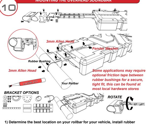
bushings on the rollbar, ensure there is ample head space 2) Apply supplied Loc-Tight to allen bolt tips, let dry for 20 minutes 3) Wrap C-clamp around rollbar, hand tighten the allen-head bolts 4) Insert left/right slide rails into REFLEX Soundbar, some vehicles will require
