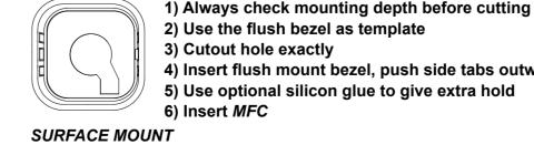
2) Use the flush bezel as template 3) Cutout hole exactly 4) Insert flush mount bezel, push side tabs outwards 5) Use optional silicon glue to give extra hold
