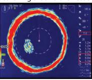
Searching around the vessel Reflected echo from seabed
