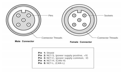
Figure 3 – NMEA 2000<sup>®</sup> Connector Face Views
